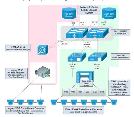
The "Green Zone" consists of videoNEXT's video surveillance management and analytic software running on a Cisco's UCS/Nexus compute infrastructure using a dedicated NetApp E-Series storage system. The Green Zone provides for state of the art video management software and analytic capacities combined with an import/parsing mechanism that
